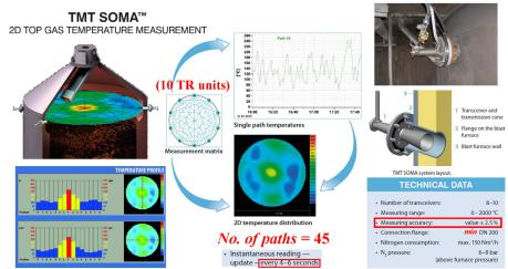
Fig.3. TMT's 2D top gas temperature measurement<sup>(2)</sup>.
