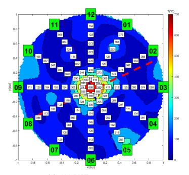
Fig.13. Gas temperature measurement result in CSC #4 BF.
