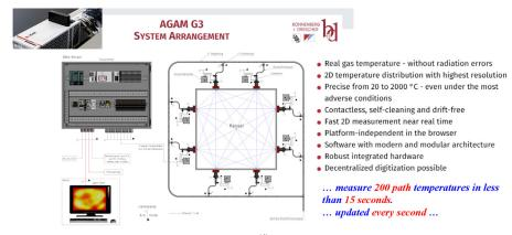
Fig.4. B&D's acoustic gas temperature measurement system <sup>(4)</sup>.
