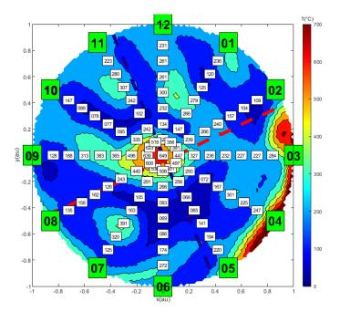
Fig.14. A channeling phenomenon observed on the acoustic gas temperature measurement system close to the furnace wall.
