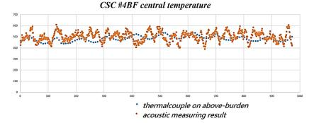
Fig.15. Trend chart of CSC #4BF central temperature.
