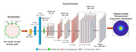
Fig.9. A deep-learning-based reconstructing method <sup>(11)</sup>.
