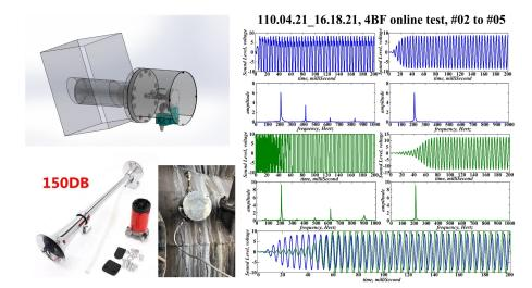
Fig.11. A sound wave transceiver designed and tested in the study.
